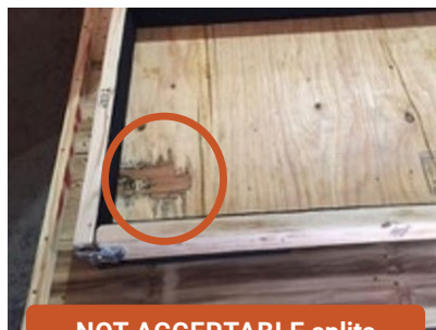
NOT ACCEPTABLE splits (caster location with no metal)
