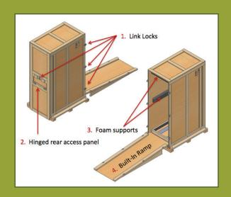
Similarly, correct foam design and placement or specialty hold down brackets or blocking can hold the rack in place during shipping and ease its removal. Keeping track of ways to prevent hardware, straps and blocking from being discarded or lost is imperative.
